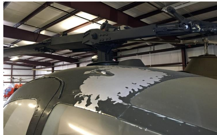
In addition to repainting, the aircraft's plexiglass windshields are badly oxidized and no longer clear. With care, all the windows will be restored to their original clarity.
