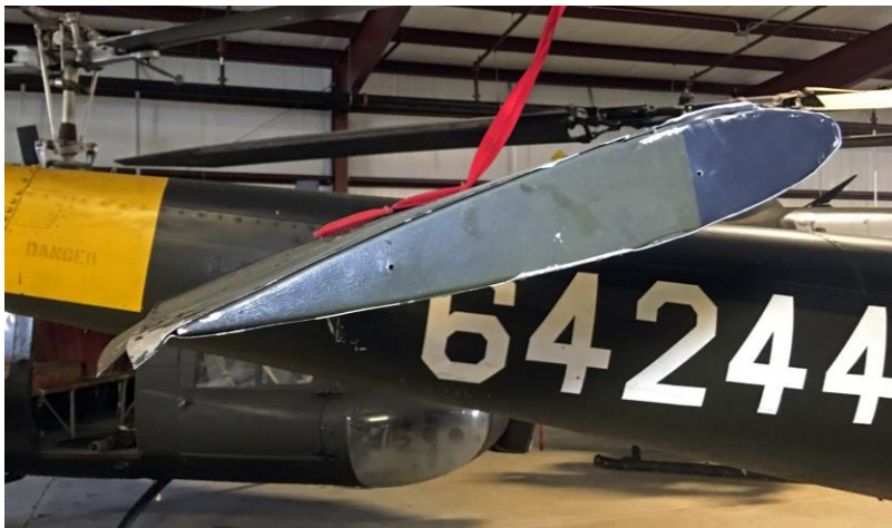
The aircraft needs some minor repairs in various locations, to include the right-side stabilizer fin with dents and smashed metal.
