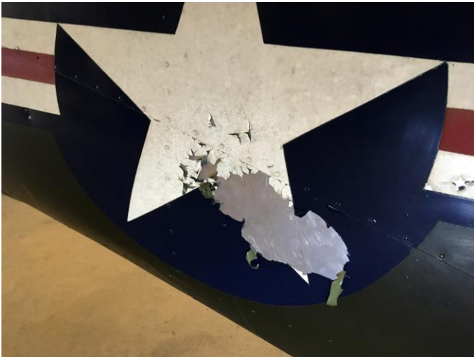
Time has taken a toll on the fuselage, as the aging paint shrinks, cracks and flakes off the metallic exterior skin.
