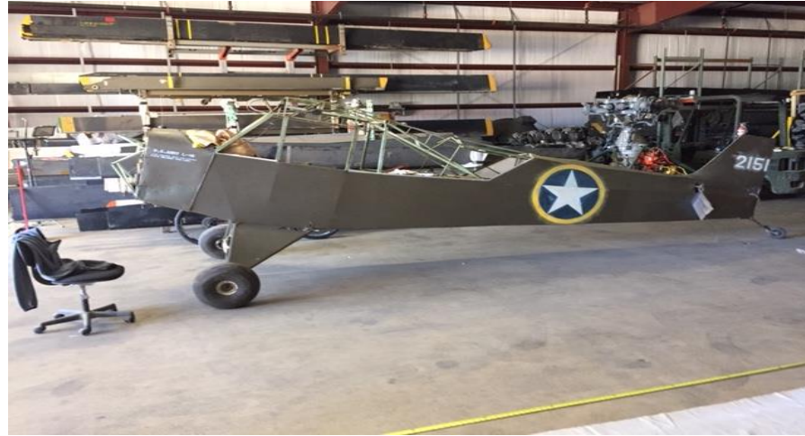
In Restoration L-4
